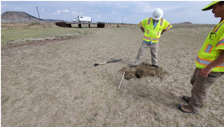
Photo 2. Wetland 1, looking northwest at SP2 (upland point) towards US 24. Upland area close to wetland boundary (photo left), soils and hydrology failed but vegetation was still considered hydrophytic. Site heavily grazed and disturbed by livestock.
